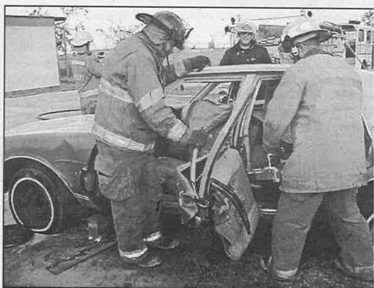
Students receive instruction on how to remove the car doors to extract a trapped passenger. To keep the car from moving, firefighters will let the air out of the tires and place blocks under them.
